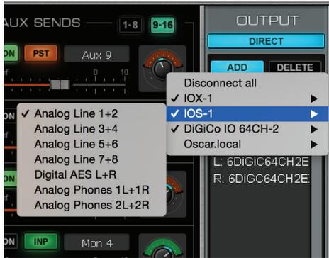
(a) Open the Direct window to assign the channel to I/Os. Add and delete device assignments here.
