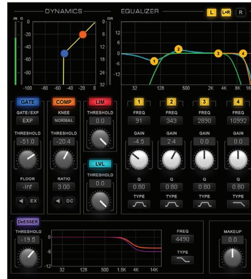
The same plugin, along with an EQ processor, in the Main section
