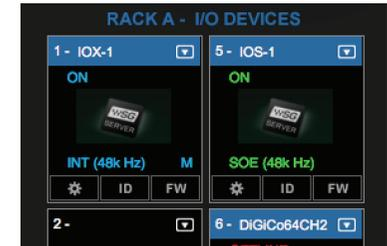
Click the down arrow on the right side of a device slot, then use the drop-down menu to add or remove devices. Up to 8 I/Os can be assigned to each rack.
