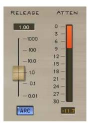
5 - Leave the ARC<sup>™</sup> (Auto-Release Control) engaged at all times unless you have a very specific type of limiter behavior, such as pumping or distortion effects. ARC calculates the release time every sample for optimum level with minimum artifacts. For nearly every possible source, ARC will outperform a fixed release time.
