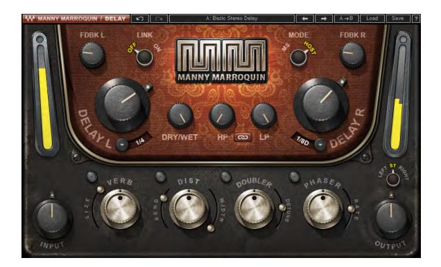
**INPUT** controls the level into the plugin. Range: -18 – 18 dB
