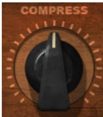
**COMPRESS** controls the amount of compression applied to the signal. (*Contours 1 & 2 only*)
