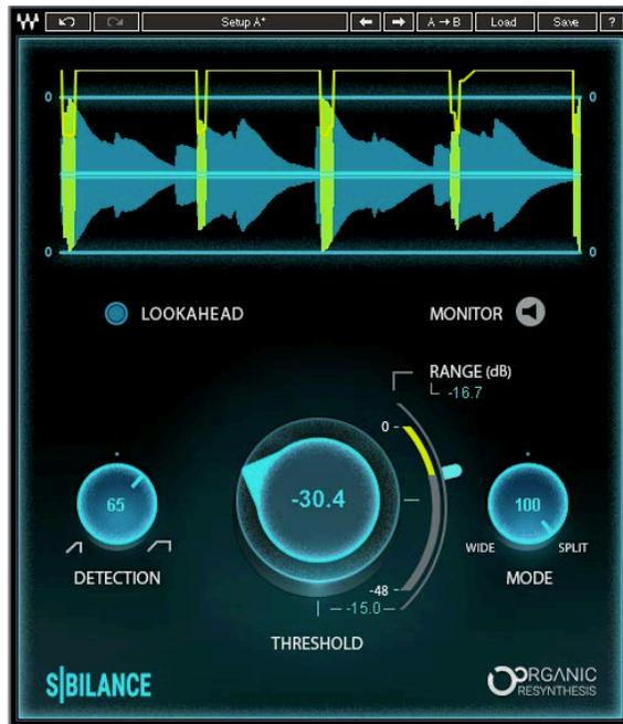
Latency for these components is determined by the sample rate and Lookahead setting.
