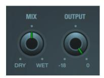
Controls the output mix between the input signal (dry) and the generated subs signal (wet). When sending the generated subs directly to an LFE channel, set Mix to 100% wet. Similarly, when using Submarine as an aux send, set Mix to 100%.
