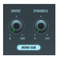
Drive adds a small amount of harmonic distortion to the sub signal. These even harmonics help the generated subs stick to the original signal. Generally, the greater the drive, the more dynamic the subs sound. Start at the default setting of 0 (zero) and slowly increase the Drive until you hear the subs get warmer and more glued to the other mix elements. At very high settings you may hear the distortion itself. Normally, you will set the subs generators before adjusting the drive.
