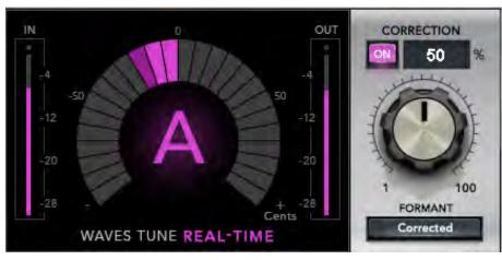
Example 2: Correction knob is set to 50%. The meter shows 20 cents pitch down.
