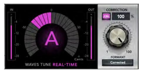
Example 1: Correction knob is set to 100%. The meter shows 40 cents pitch down.
