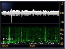
The X-Crackle Scope provides visual feedback for the last 10 seconds of processing history. The incoming waveform is shown in gray at the top. The bottom, green waveform shows frequency domain data in the y-axis and time across the x-axis. Higher Threshold values yield more green data in the scope.
