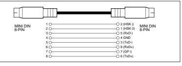
• 8-pin system peripheral cable.
