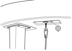
Left of the rear leg on the bottom of the main unit, when viewed from front
