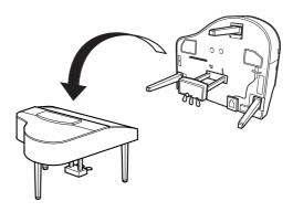
5 Set the voltage selector and connect the power cord.
