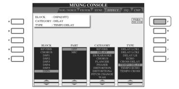
10 If you have selected one of the DSP 2–5 effect blocks in step 5: You can edit its standard parameters as well as its variation parameter. To select the standard type of parameters, press the [B] button. To select its variation parameter, press the [E] button.
