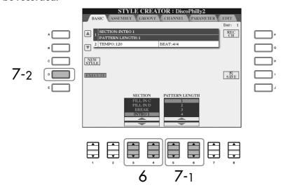
Use the [5 ▲ ▼]/[6 ▲ ▼] buttons to determine the length (number of measures) of the selected section.
