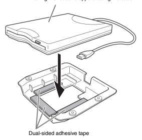
2 Fold the USB cable inside the case as shown.
