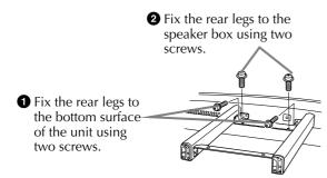
If the screw holes do not align, loosen the other screws and adjust the position of the rear legs.
