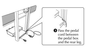
Make sure that the pedal box lays flat, with no gap between itself and the floor, then affix the pedal box using two screws.
