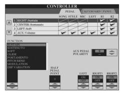
In addition to the footswitch or foot controller, the three piano pedals installed to the instrument (Right, Center and Left pedals) can also be assigned to various functions here. The following explanations cover the related operations and assignable functions (parameters).
