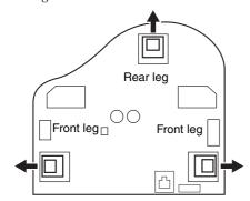
• Install and tighten four screws on each leg, starting with one of the front legs.
