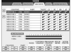
The explanations here apply to the RECEIVE display to be called up in step 4 of the "Basic Operation" on page 196. This determines which parts will receive MIDI data and over which MIDI channels the data will be received.
