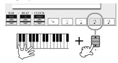
While holding the C3, E3, G3 and C4 keys on the keyboard, press the [7 ▲ ▼] button, and successively press the [5 ▲ ▼] button.
