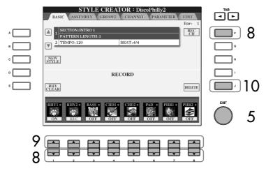
Call up the Voice Selection display by using the [1 ▲]–[8 ▲] buttons and select the desired Voice for the corresponding recording channels.
