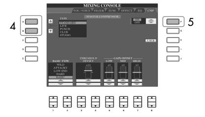
5 Press the [F] button to set the Master Compressor to ON.
