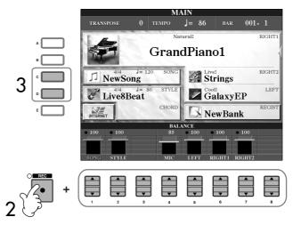
3 Use the [C]/[D] buttons to select the desired part for the channel to be recorded.
