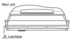
To prevent the key cover from accidentally opening during assembly, press down on the key cover, making sure that the sheet (shown) remain in place.
