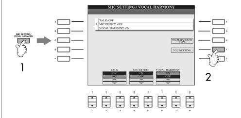
Press the [I] (MIC SETTING) button to call up the MICROPHONE SETTING display.
