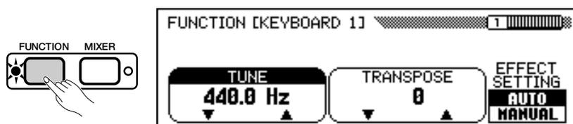
**2** Select the page of the desired function by using the PAGE [◀] [▶] buttons. The Function mode contains a total of seventeen pages.
