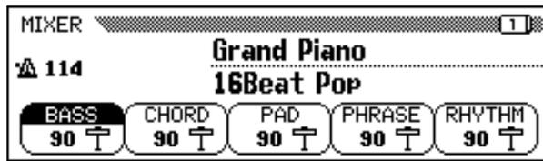
Select the desired part by pressing **BASS**, **CHORD**, **PAD**, **PHRASE**, or **RHYTHM** and set the value by using the data dial or [-/+ ] buttons. The value changes in units of two. You can also select several parts and adjust their volume settings simultaneously. To reset the value to the basic setting of 90, simultaneously press the [-/+ ] buttons.
