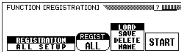
To save or load the data of **REGISTRATION**, first set the **REGIST** (Registration number) parameter. When saving, press the **REGIST** button to select the desired Registration file number from **ALL** or **A-1 – E-4** to save to disk. When loading, select the internal destination location from **ALL** or **A-1 – E-4**.
