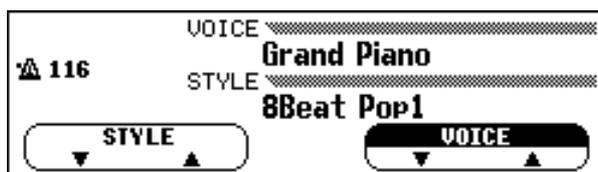
For functions or parameters that have ▼ and ▲ or ◀ and ▶ indications, you can reset the value to its basic value by simultaneously pressing both LCD buttons (or both [-/+ ] buttons).
