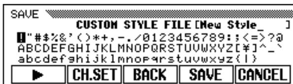
Your custom styles must be stored to internal memory before they can be saved to disk (see step 10 of the basic custom style recording procedure). If a custom style has not been stored and you attempt to save it to disk, the “**Please store to memory before saving to disk**” alert display will appear. If this happens press **OK** to return to the previous display (CUSTOM STYLE display page 3), store the custom style, then try saving again.
