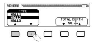
You can also select the Type by pressing **TYPE** (it is highlighted) and using the data dial or [-/+] buttons.
