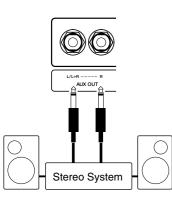
By connecting audio cables to the jacks as shown below, output the sound of the CVP-94/ 92 to a stereo system, amplifier, mixing console, or recording equipment. Set the [MAS-TER VOLUME] of the CVP-94/92 to around the middle position and adjust the volume level from the connected equipment.
