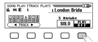
Select a track, then press and highlight the **SOLO** LCD button to hear only the selected track. Press the **SOLO** LCD button again to cancel the Solo function.
