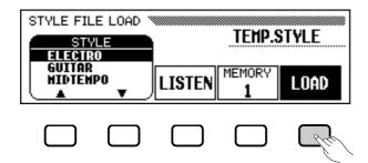
It is not necessary to select a memory number when ALL LOAD is selected in step 1. Simply press **OK** to load or **CANCEL** to abort.
