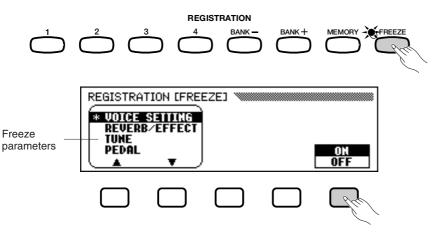
Parameters set to Freeze ON appear with an asterisk (\*), and "ON" (in the **ON/OFF** section) is highlighted.
