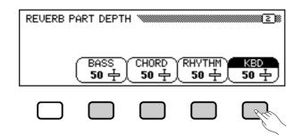
Select the desired part by using the **BASS**, **CHORD**, **RHYTHM** and **KBD** (keyboard) in the REVERB PART DEPTH display. You can also select several parts and adjust their settings simultaneously.
