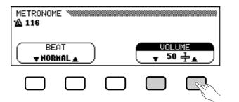
Adjust the volume by selecting **DOLUME**  $\checkmark$  (it is highlighted) and using the data dial or [-/+] buttons.
