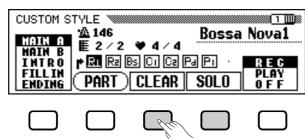
Another useful recording aid is the **SOLO** LCD button: when this button is pressed and highlighted, only the selected part will sound. Press the **SOLO** button again to turn the solo function off and hear the entire style.
