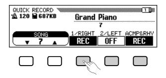
When a part is set to **REC** (record enable), recording is set to stand-by and automatically starts when you play the keyboard.
