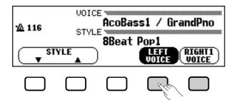
After pressing **LEFT DOICE** or **RIGHT1 DOICE** (it is highlighted), select the voice in the normal way.
