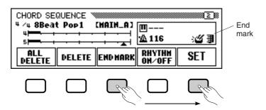
Finally, press the **[REC]** button and a "Save recorded data?" message will appear. Press **YES** to store the recorded data and automatically leave the Chord Sequence function; the display returns to the SONG PLAY display. To leave without saving the data, press **NO**. To continue editing the sequence without saving the data, press **CANCEL**.
