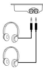
To use headphones, connect them to one of the **[PHONES]** jacks (standard 1/4" phone jacks). The internal speaker system of the CVP-94/92 is automatically shut off when a pair of headphones are connected. Two people can enjoy the sound together by connecting two pairs of headphones to the two available terminals.
