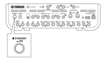
2 Connect the DC plug of the included AC power adaptor to the DC IN jack on the rear panel. To prevent the cord from being unplugged accidentally, wrap the cord around the cable clip and secure it.
