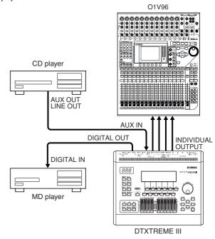
The OUTPUT (L/MONO and R) and INDIVIDUAL OUT-PUT (1 to 6) jacks produce line level audio signals regardless of whether headphones are connected or not. These jacks are mono phone type. To make audio connections via these jacks, use cables with a mono phone plug for the DTXTREME III and an appropriate plug for the other device.
