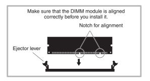
4-1 Press the ejector levers to the outside of the socket.
