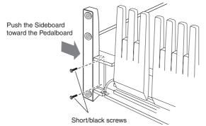
**3-3** Stand the Pedalboard after securing the screws.
