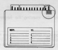
NOTE: If you wish to preserve the contents of a Registration Pack, simply break the tab on top of the pack. When this tab is missing, the WRITE operation cannot be performed and therefore the contents of the Registration Pack cannot be erased.
