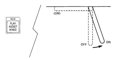
The KNEE LEVER (located beneath the keyboards) can be used to turn the PLAY ASSIST functions "ON" or "OFF," thus enabling a variety of voicings in any given song. To operate, press the PLAY ASSIST (KNEE) button (located in the SUSTAIN section) and then move the KNEE LEVER into a vertical position, placing it to the right of your right knee.
