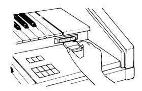
When the Registration Pack is properly inserted, the MEMORY READY lamp will flash briefly and then remain on, indicating that the Memory is now ready to receive the information from the Electone™.
