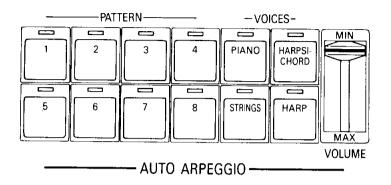
This function automatically produces arpeggios (a series of notes, most often derived from a chord, in which one note at a time is played, in succession, from the lowest note to the highest) providing a sparkling background accompaniment. Due to technological advancement, what once took many hours of practice to be able to execute can now be accomplished automatically by simply holding one or more notes on the Lower Keyboard.
