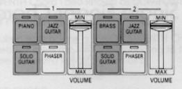
As you can see by the above illustration, the Rhythmic Chord function is divided into two independent groups, (called Voice 1 and Voice 2), enabling two different accompaniment patterns to be simultaneously produced. Each section incorporates three different instruments. Only one instrument per group may be used at any given time.
