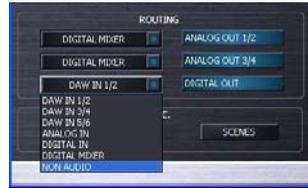
\* For the DIGITAL OUT jack, you can select "NON AUDIO" (as shown above). In this case, AC3 and DTS data will be transmitted only via the digital output.
