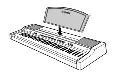
The YPP-100 is supplied with a music rest that can be attached to the instrument by inserting it into the slot at the rear of the control panel.
