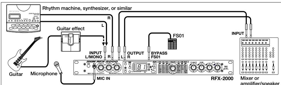
This is an example for inserting the RFX-2000 between the sound source such as a microphone or instrument and a playback system or multi-track recorder (MTR). A stereo source should be connected to the INPUT L/MONO and R jacks. A mono source should be connected to the L/MONO jack only.
