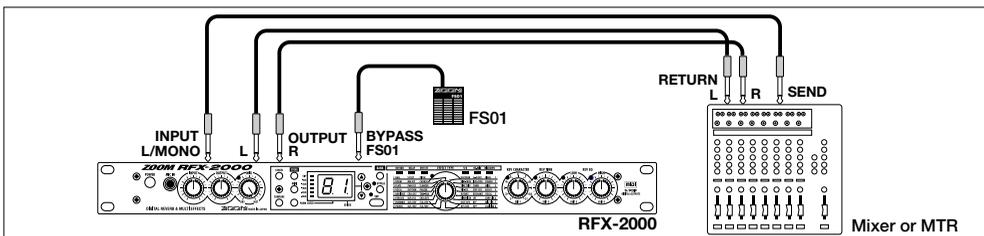
This is an example for connecting the RFX-2000 to the send/return jacks of a mixer or multi-track recorder. Connect the send jack of the mixer or MTR to the INPUT L/MONO jack of the RFX-2000, and connect the OUTPUT L/R jacks of the RFX-2000 to the return jacks (or the stereo line input jacks) of the mixer or MTR.
