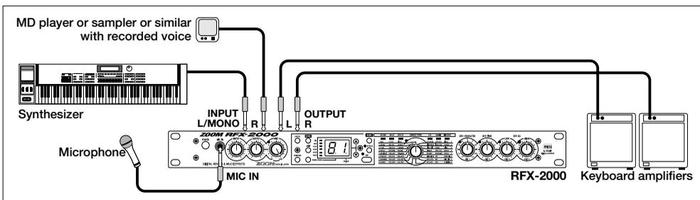
This is a connection example for using the VOCODER effect from the SFX bank. Connect a dynamic microphone to the front-panel MIC IN jack on the RFX-2000. Connect a synthesizer or other instrument to the rear-panel INPUT L/MONO jack. You can then use the mike to vary the
