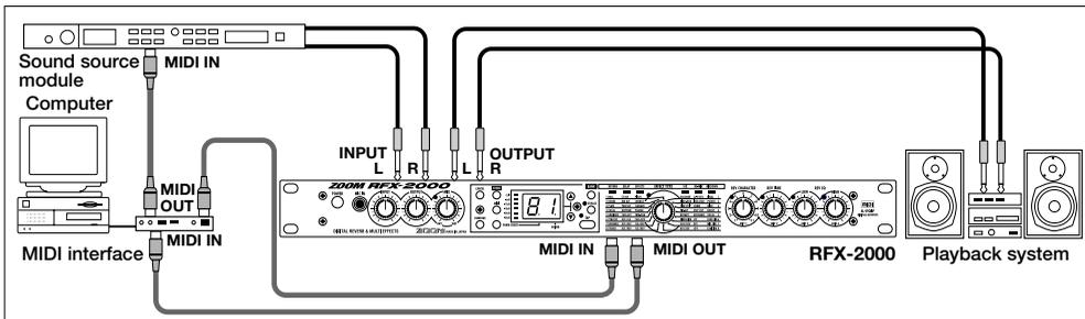
The supplied software can be used to edit the patches of the RFX-2000, switch the patches in conjunction with other sequencer software, and to control patch switching and make parameter changes. To enable these functions, make connections as shown above.
